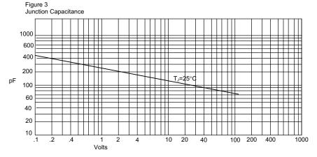
Junction Capacitance - pF versus Reverse Voltage - Volts
